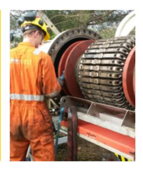
Active Speed Control • Multi-diameter inspection • Bidirectional inspection • Low-flow solutions • Spatial mapping and strain analysis Small diameter pipelines • Low friction tools • Brushless design for traverse of umbilicals • Short radius bends • Illegal Hot Taps
