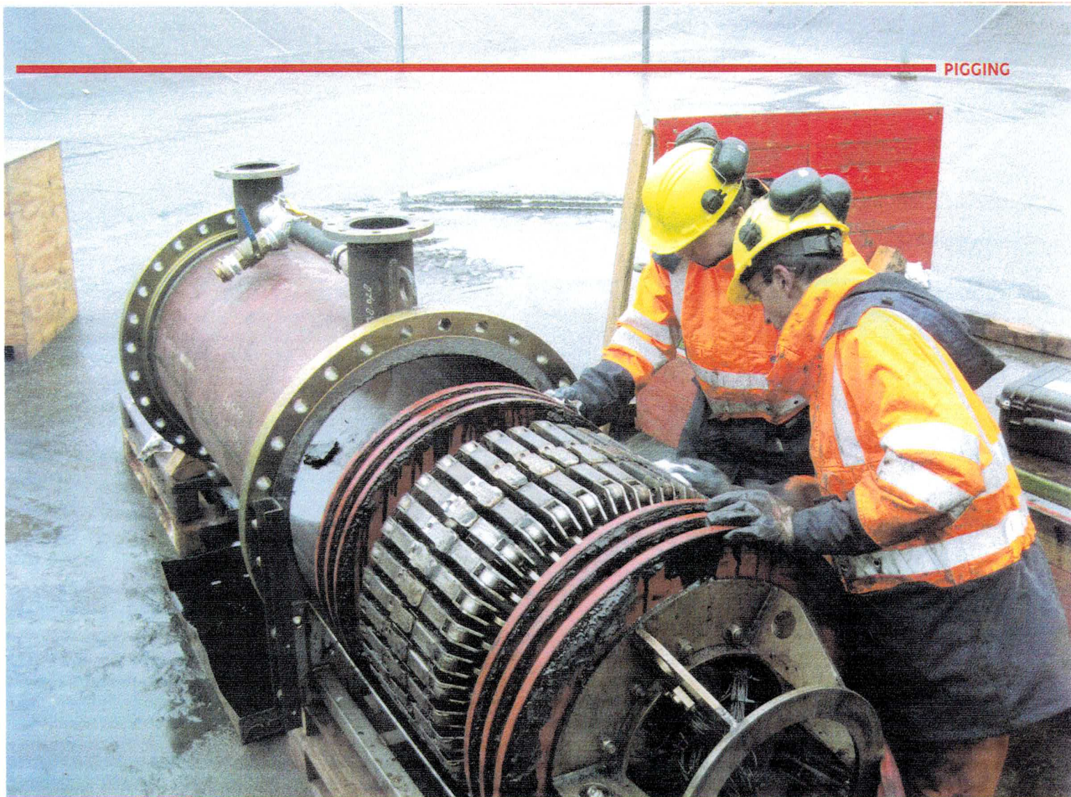
A 30 inch bi-directional tool with temporary pipe spool upon completion of first inspection run.
